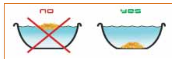
Pellets floating and sinking - Test for pellet quality
